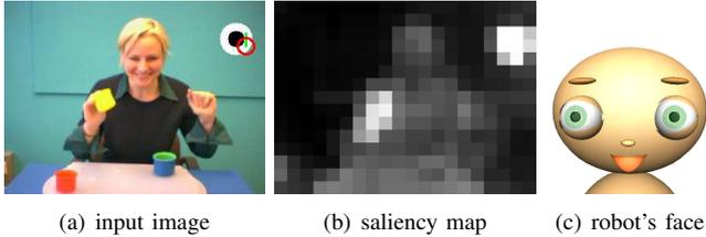
Fig. 2. A scene with disturbance (a black and white circle) superimposed in the image, which attracts the robot's attention more than the yellow cup because of the highly contrasted intensity and the motion
